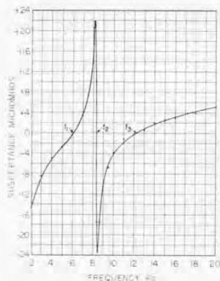
Figure 8. Susceptance variation of a 5-henry inductor at frequencies where distributed capacitance produces resonance effects.
